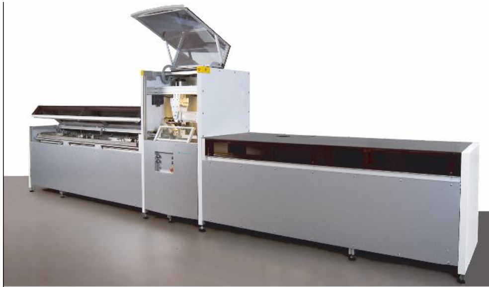
Figure 2.3 :Front view of the Itrax core scanner with open hoods (Croudace et al, 2006).
