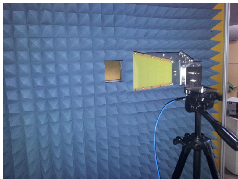
Figure 5.6 : The location of the FSS in the test setup for Ku Band
