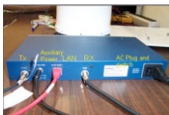
Figure 2.3 : Indoor equipment for VSAT [14].
