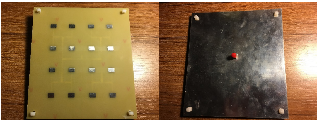
Figure 4.5 : Antenna view after connection two sides with handcuffs.
