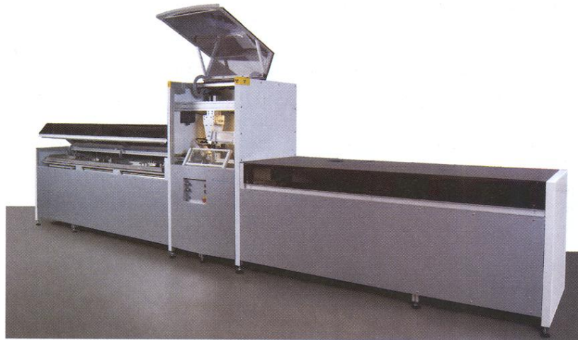
Fig 2.3: Front view of the Itrax core-scanner with open hoods
