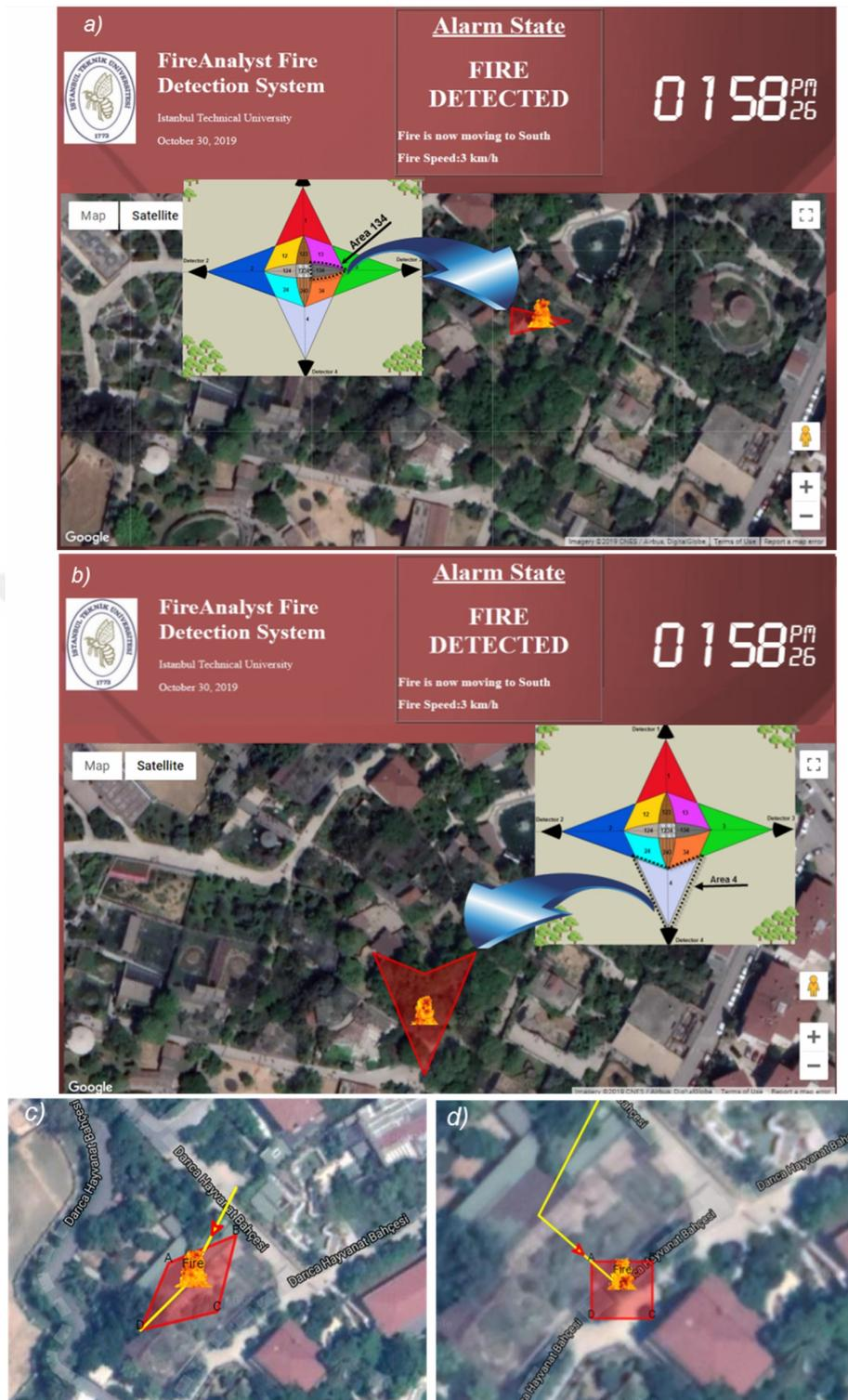
**Figure 5.4 :** Created fire area polygon samples on Map for: (a) Case: 134 polygon; (b) Case: 4 polygon; (c) Case: 12 polygon; (c) Case: 1234 polygon.
