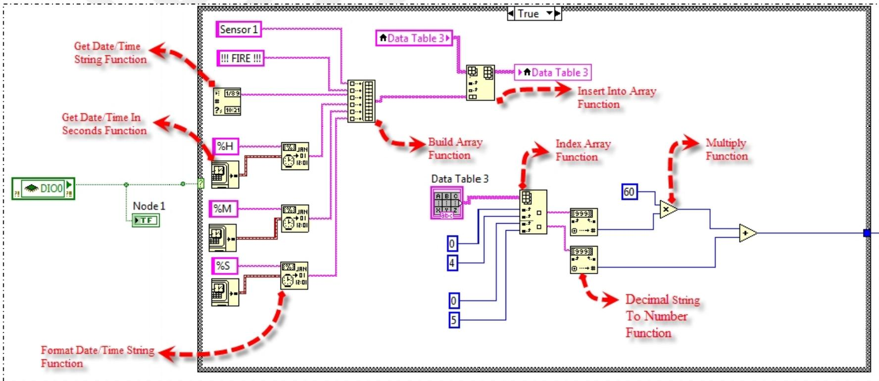
Figure 4.5 : A True-False case structure.
