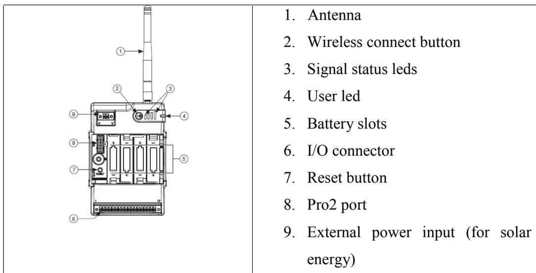
**Figure 2.1** : Wireless sensor node interface , adapted from National Instruments Corp. (2013).
