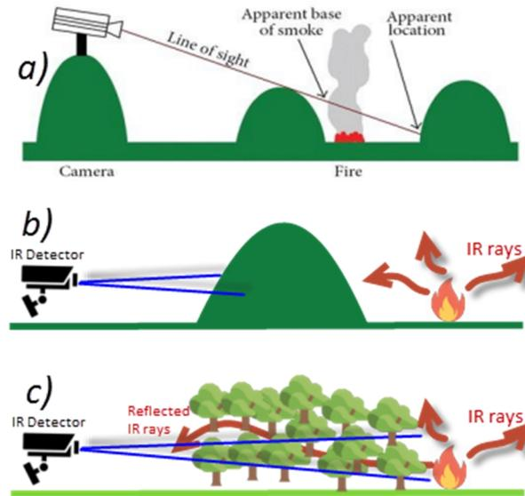
**Figure 6.2 :** Flame detection handicaps: (a) Location error, adapted from Mathews (2010); (b) Rugged terrain case; (c) Trees case.
