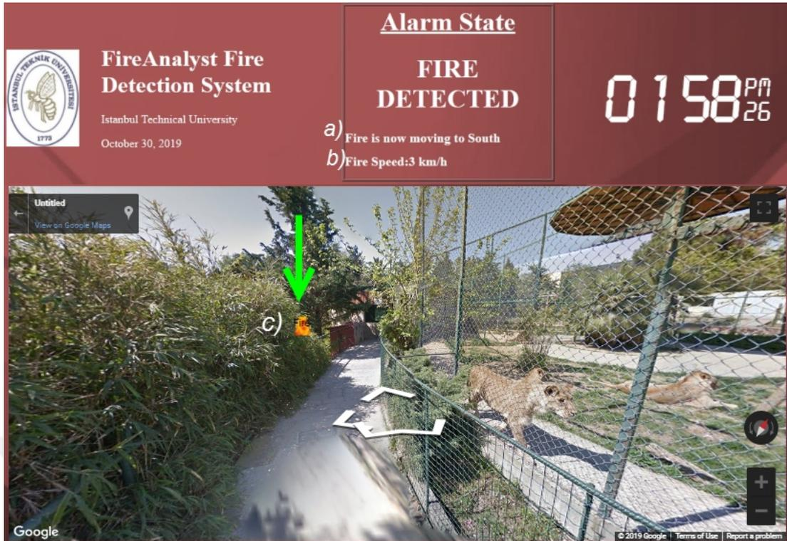
**Figure 1.1 :** FireAnalyst Map Portal: (a) State of fire, (b) Fire behavior outputs, (c) Simulation of real-time estimated geolocation of fire.
