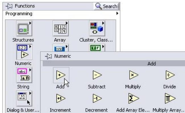
**Figure 4.4 :** Type of functions blocks.
