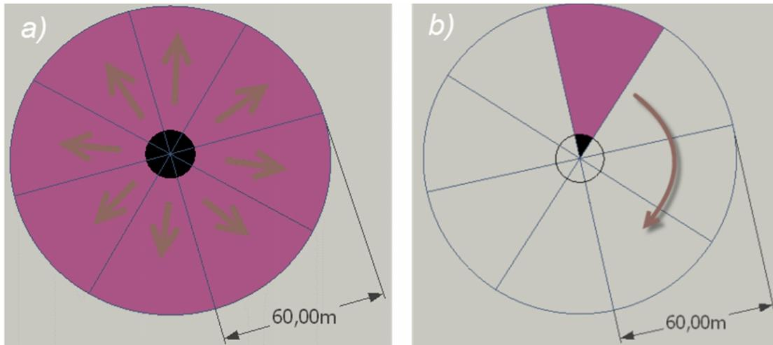
**Figure 3.1 :** DBOC Geometry: (a) 8 fixed detectors in DBOC geometry; (b) spinning detector in DBOC geometry.
