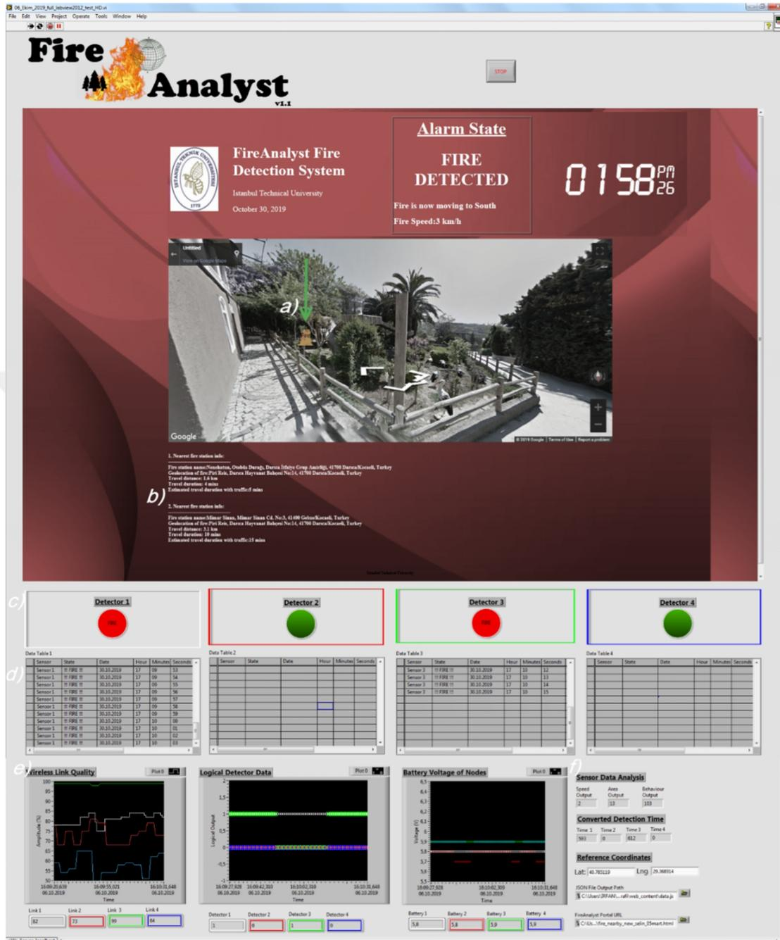
**Figure 4.8 :** FireAnalyst Front Panel View: (a) Detected fire geolocation; (b) Nearby fire stations discovered; (c) Indicator LEDs; (d) Data tables of WSN nodes ; (e) Info dashboards for WSN nodes; (f) Admin section.
