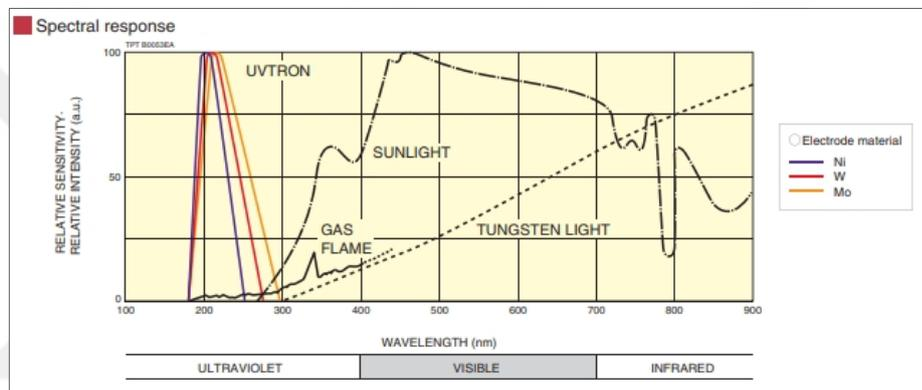
**Figure 2.6 :** Spectral response of nanophotonic flame detector, adapted from Uvtron (2018).
