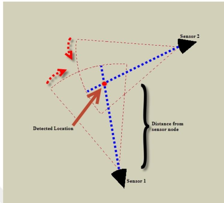
**Figure 3.6 :** Intersection of boundaries in detection area.
