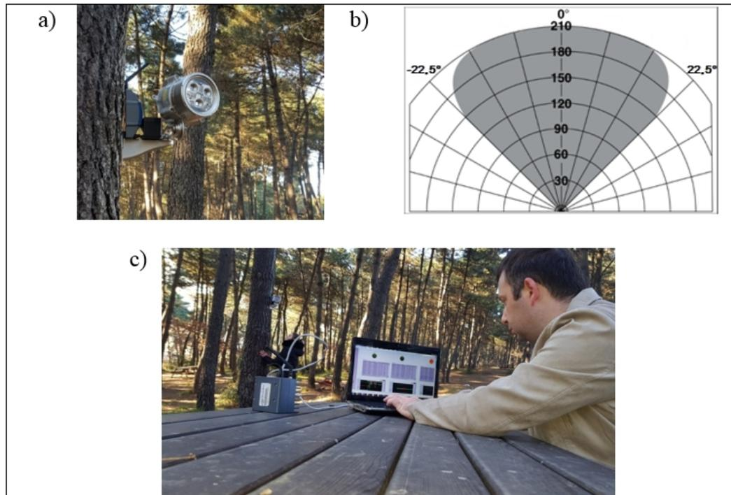
**Figure 1.4 :** System implementation: (a) Multi-IR detector and transmitter, (b) Cone of vision of detectors (ft vs. degree), (c) Implementation of monitoring system.
