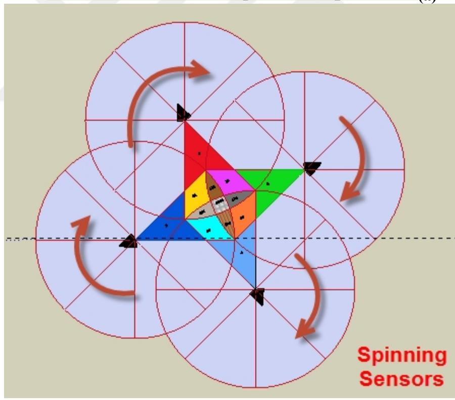
Figure A.1 : Mesh Network of Spinning Sensor Geometries: (a) Fixed Sensor Geometry with 16 Sensors (b) Spinning Sensor Geometry with 4 Sensors.
