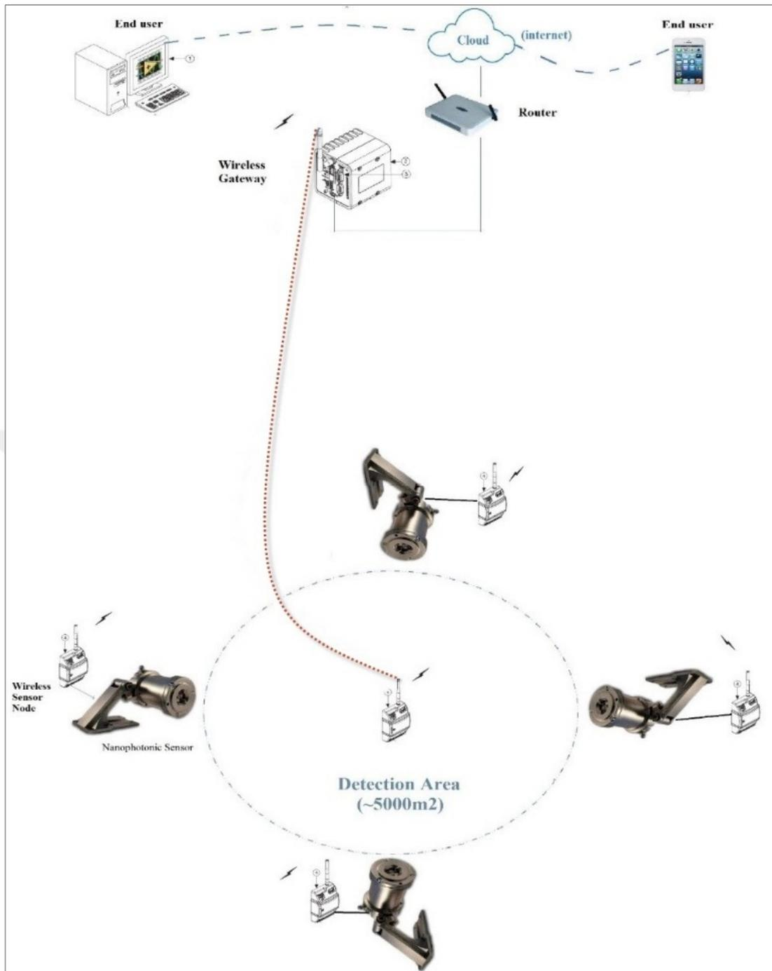
**Figure 1.3 :** Architecture of the Fire Detection System.
