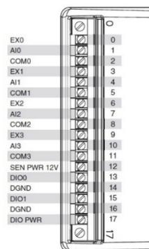
**Figure 2.2 :** Pinout characteristics of wireless nodes, adapted from National Instruments Corp. (2013).
