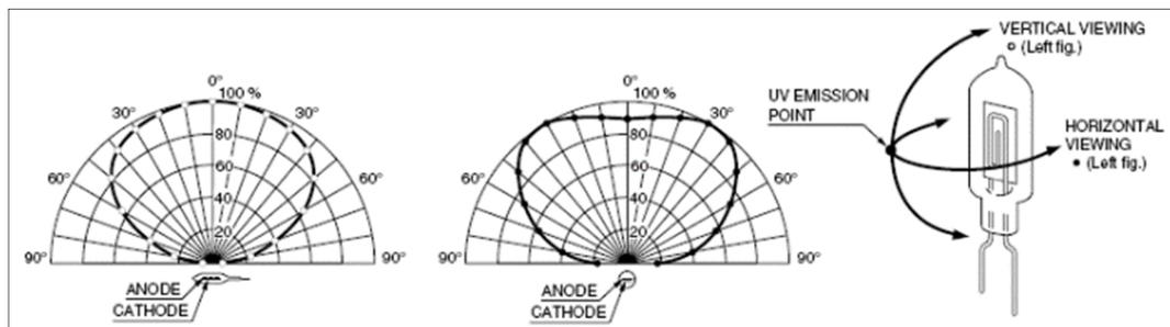
**Figure 2.7 :** Angular sensitivity (directivity) flame detector, adapted from Takex Inc. (2010).
