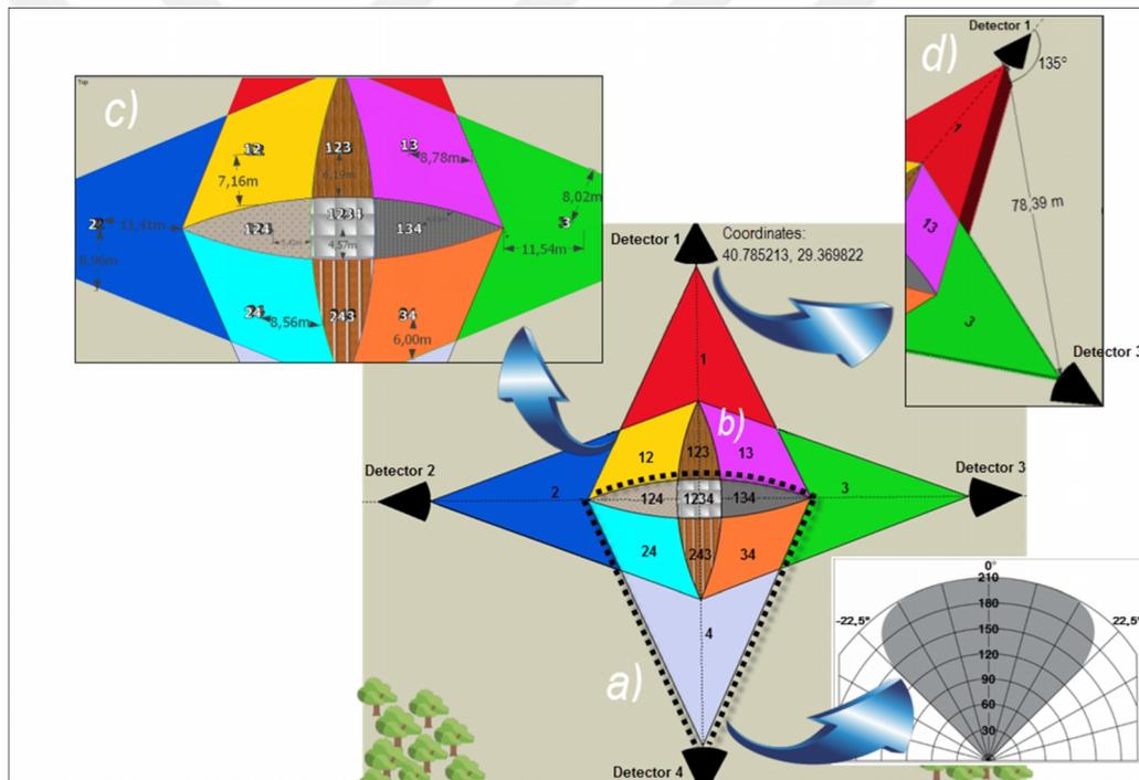
**Figure 1.5 :** Superposition of detection areas of 4 Multi-IR detectors and superposed regions: (a) Detection area of 4th detector; (b) a new and smaller superposed region labelled as 13; (c) Distances from midpoints to borders; (d) Spherical geometry parameters for auto-calculation of coordinates of the other detectors.
