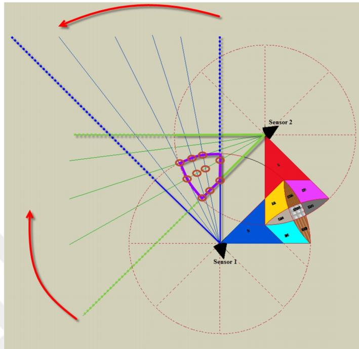
**Figure 3.5 :** Intersection of boundaries of detection areas during spinning.
