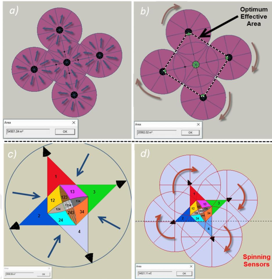
**Figure 3.2 :** Geometry types for detector positions: (a) DBOC geometry with 40 fixed sensors; (b) Created OEA by superposition of detection areas in DBOC geometry; (c) DBTC geometry with 4 fixed detectors; (d) Detection area of four spinning detectors with DBTC geometry.
