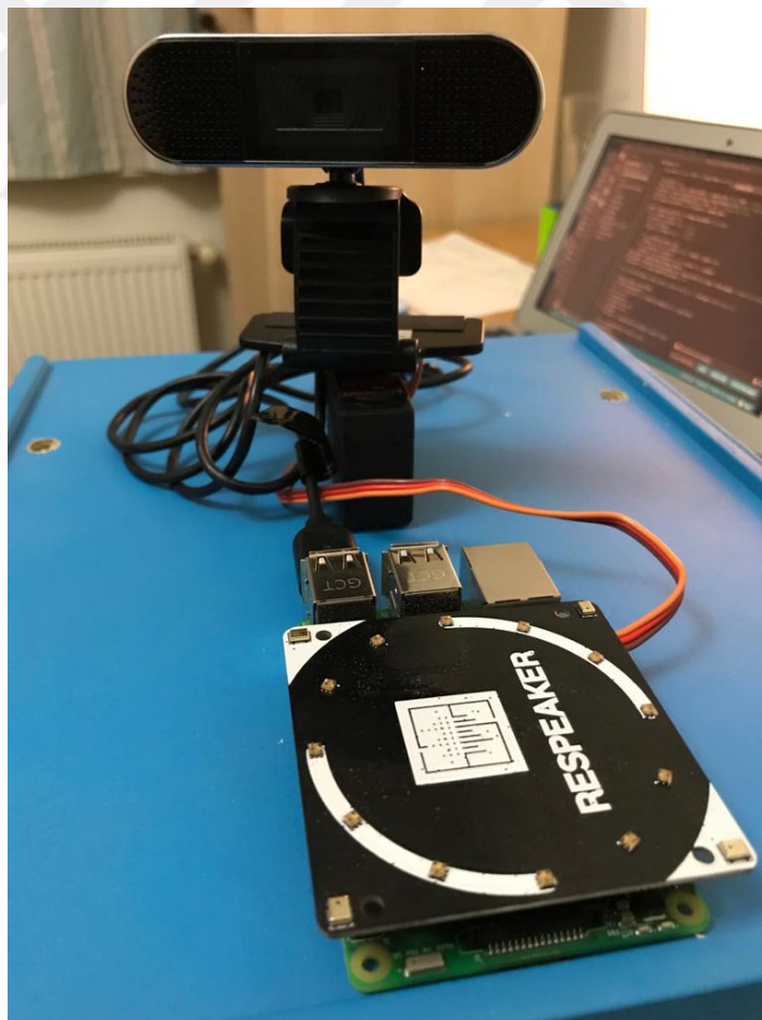
Figure 5.1 : Prototype Setup consist of a camera, Macbook Air, robot servo, Microphone array and a Raspberr Pi
