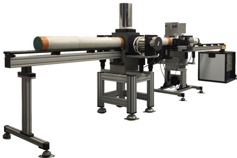
Figure 3. Geotek Multi Sensor Core Logger, MSCL
