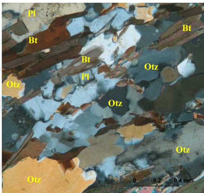
Figure 2.10: Micaschist, Sarıcakaya complex (~4.5 km north of Sarıcakaya town). Qtz: Quartz, Bt: Biotite, Pl: Plagioclase.
