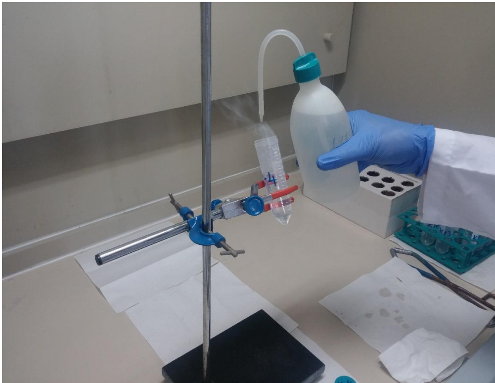
Figure 2.5 Chemical separation; acidifying
