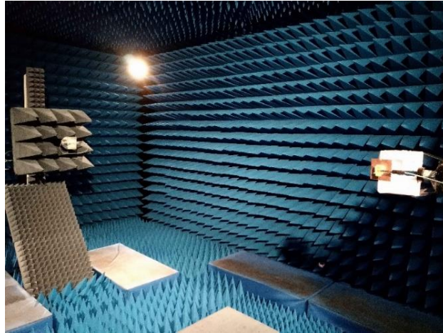
Figure 5.15: Anechoic Chamber and Far-Field Measurement for Fabricated Antenna.
