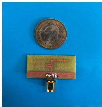
Figure 5.2: Fabricated Unit Cell Antenna.
