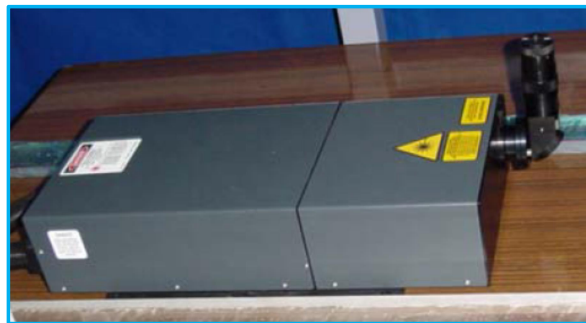
Figure 3.16. Source of a Nd. YAG Laser used in PIV experiments
