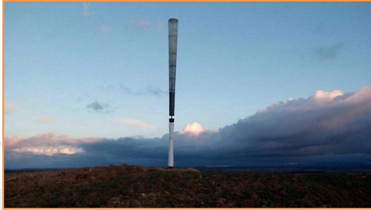
Figure 1.44. A view of vortex bladeless wind turbine generating power
