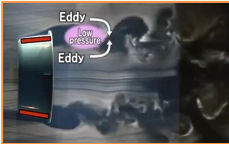
Figure 4.84. Low pressure zone resulting enhanced mass flow rate of Ohya et al. (2004) study
