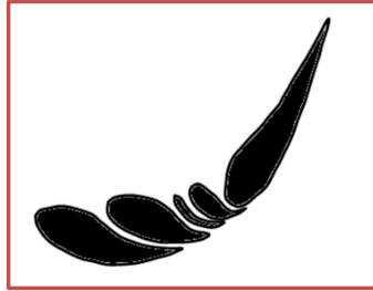
Figure 1.35. The airfoil type casing appropriate for small scale wind turbines with passive control devices (Coşoiu et al., 2013)
