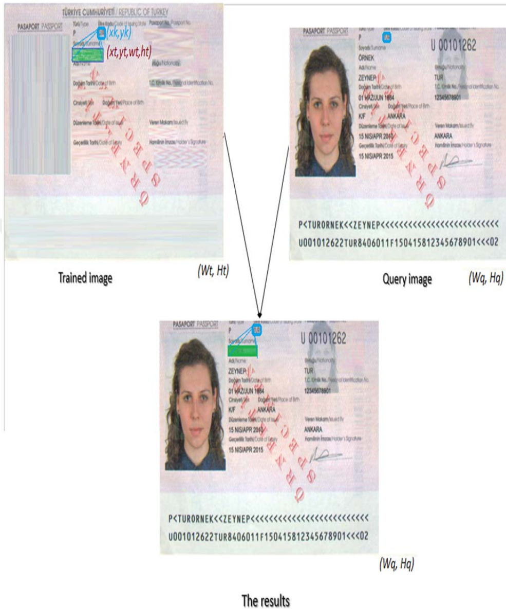
Figure 3.9. The results after applying the template matching method between the typical image and query image.
