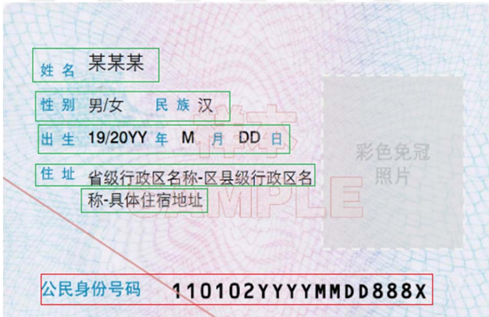
Figure 3.3. An example of merging document number label with the document number segment as one area on the text detection method.
