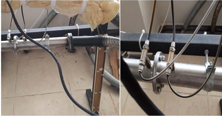
Figure 5.16. Manometer with an orifice plate
