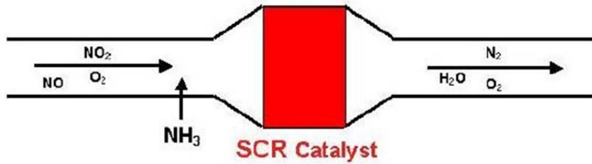
Figure 3.9. Working of SCR (Müller, 2013)
