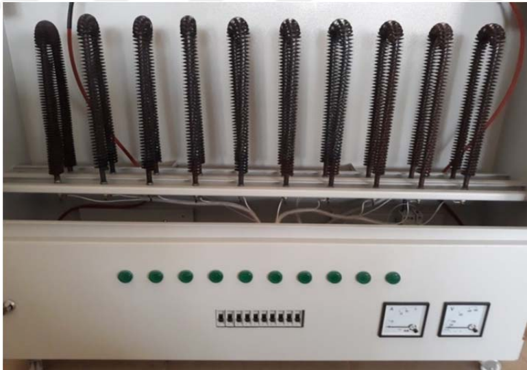
Figure 5.19 . Electric loading system
