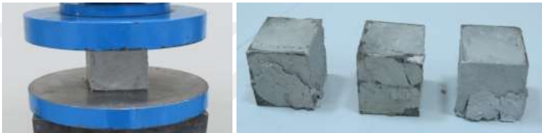
Figure 3.11 : Compressive strength test of epoxy.
