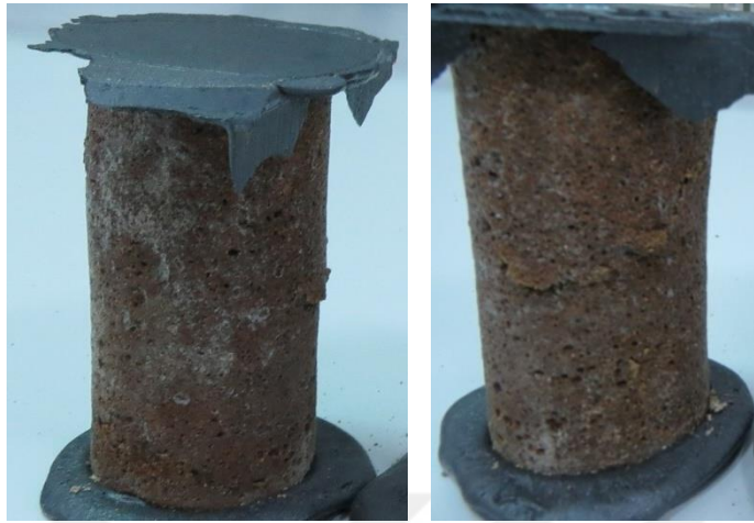
Figure 5.8 : Specimens view a) before and b) after failure
