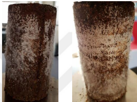
Figure 5.5 : Specimen with lime a) before and b) after test
