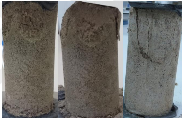
Figure 5.10 : Failure mode of specimens
