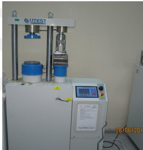
Figure 4.6 : Unconfined compressive strength test machine
