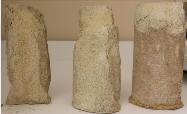
Figure 5.16 : Failure mode of specimens
