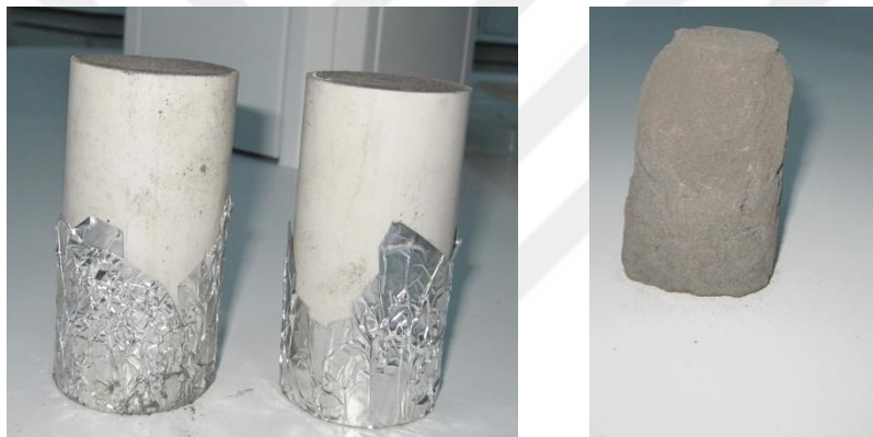
Figure 5.2 : Unmolded specimens or spread during unmolding
