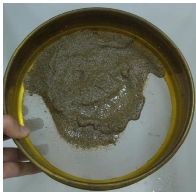
Figure 4.3 : Washing of sandy soil through sieve with diameter 74 \mu\text{m}
