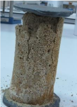
Figure 5.12 : Failure mode of specimen
