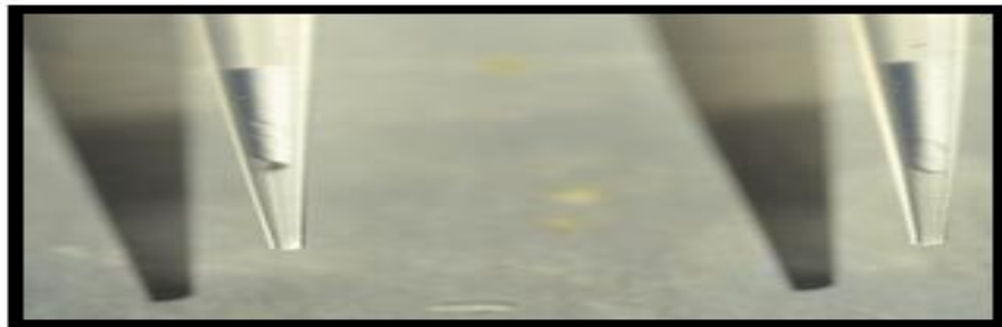
Figure 3.2 : Real images of paper extraction support material after fabrication into the pipette tips in the use of nucleic acid extraction
