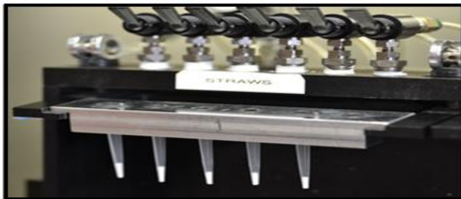
Figure 3.3 : Simple pressure manifold for using in determination of flow rates of the paper tips in order to use in lysis and extraction of HPV DNA prior to detection
