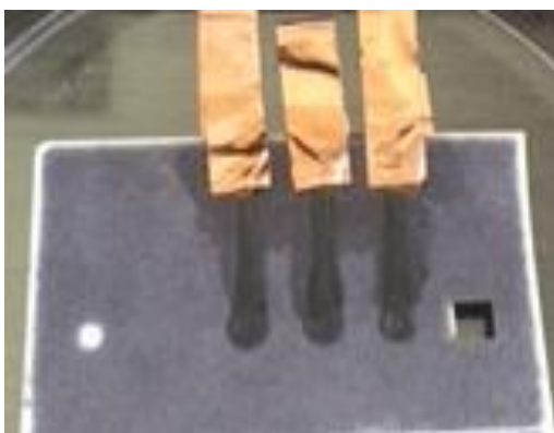
Figure 5.4 : Electrical contacts of carbon paste printed electrode
