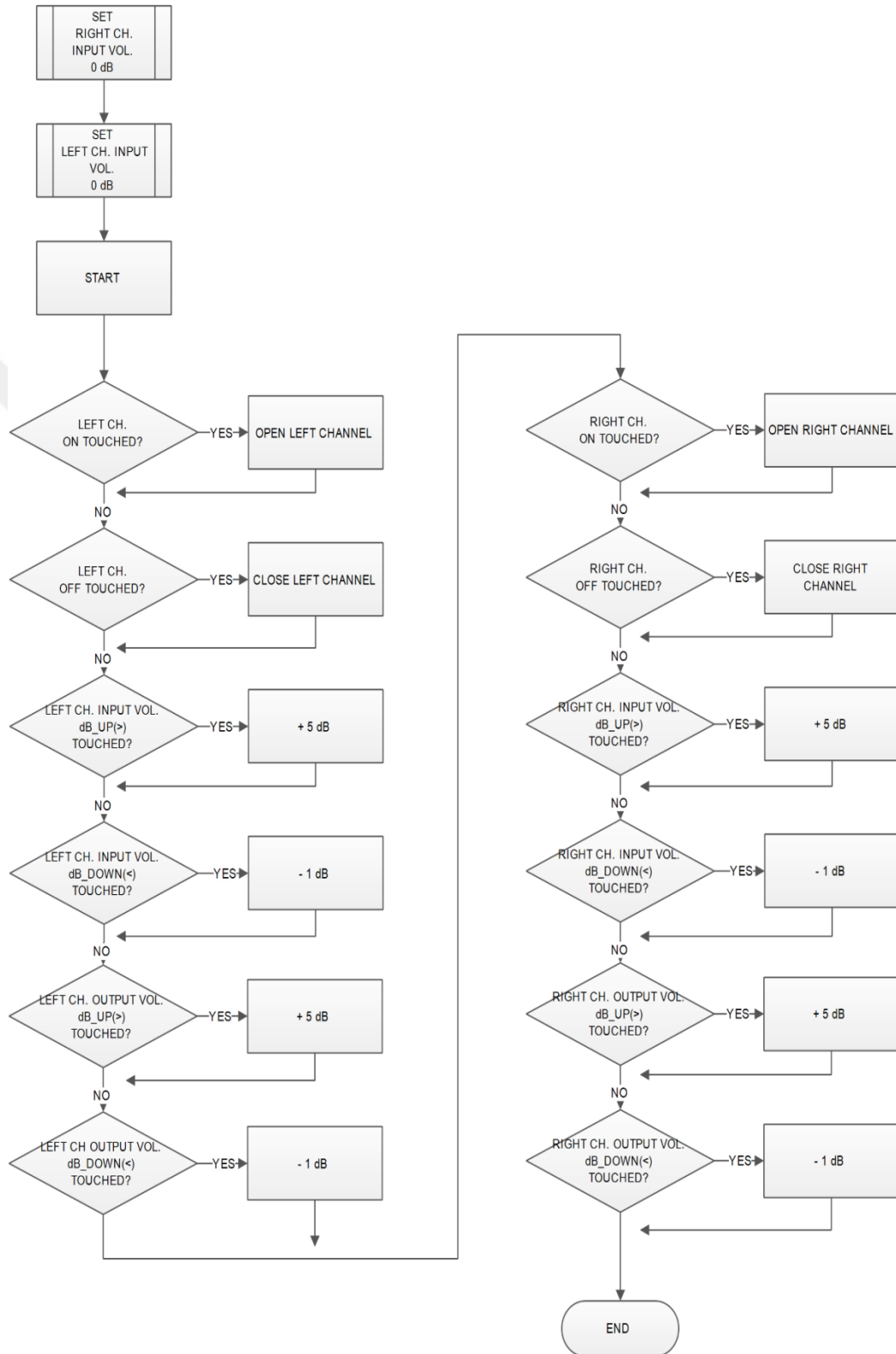
Figure 2.16: Mod 3 software flowchart.
