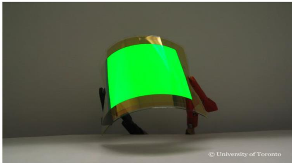
Figure 1.2 : OLED materials can be deposited on flexible substrate (URL1)
