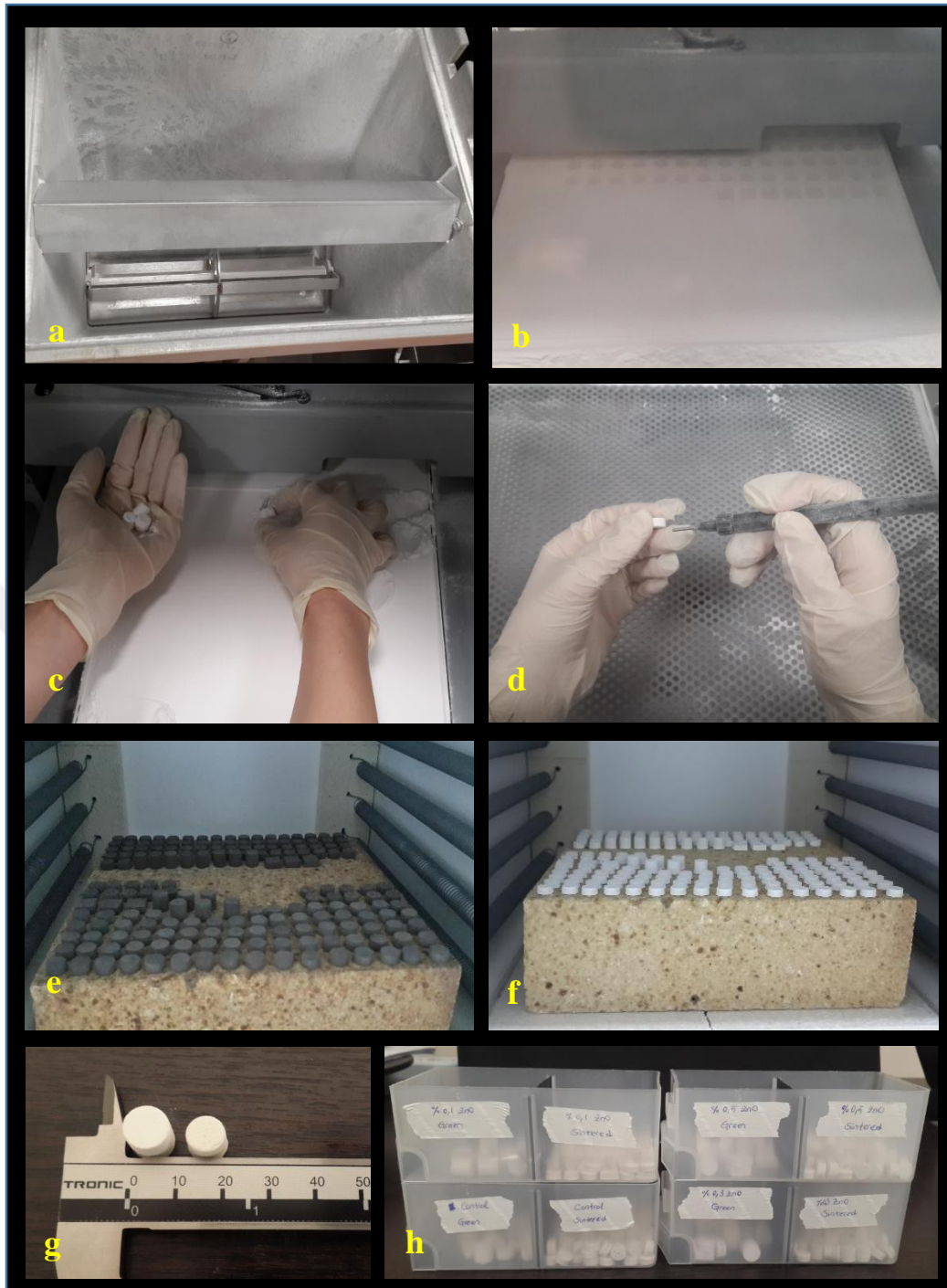
Figure 3.3 : Sample production process a. emptying and cleansing printer feeding chamber, b. printing parts with loaded powder, c. collecting samples from building area, d. depowdering loose powders by using air blowing e. pre-baked samples, f. sintered samples, g. sintered and non-sintered samples, h. all manufactured groups.
