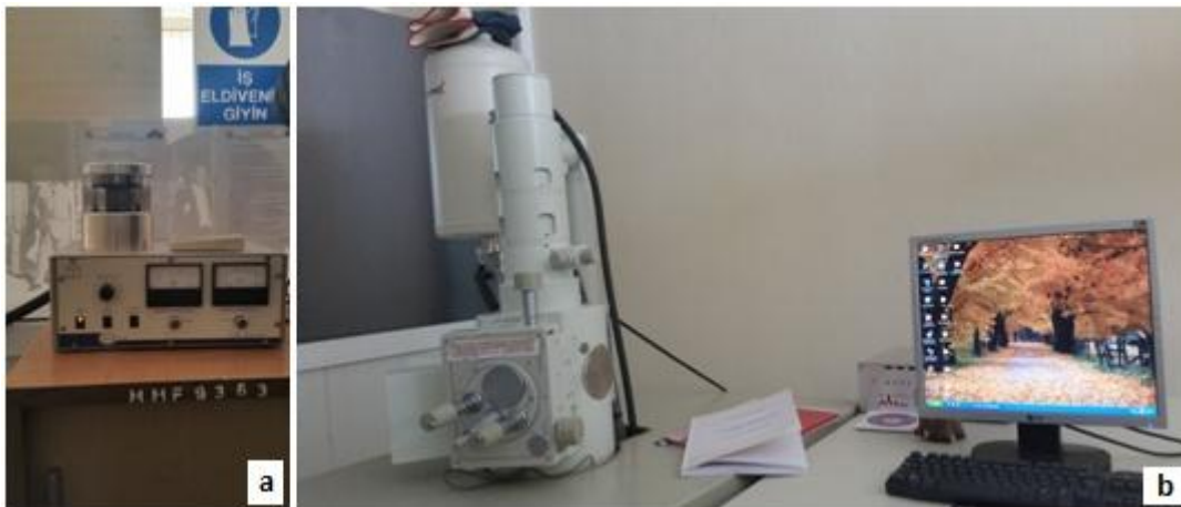
Figure 2.6: a) Sputter coating device and b) Scanning electron microscope.
