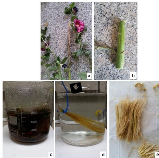
Figure 2.1: Fiber extraction process a) fresh plant, b) cleaned part of stem, c) NaOH boiling, d) warm water washing, e) chemically extracted fibers.
