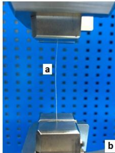
Figure 2.8: a) Mounted single fiber b) Tensile testing machine.
