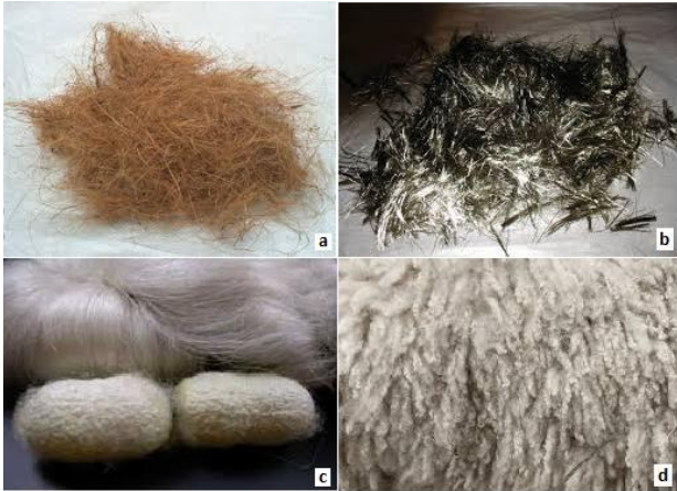
Figure 1.4: Examples of natural fibers a) plant fiber, b) basalt fiber, c) silk fiber, d) wool fiber [24].
