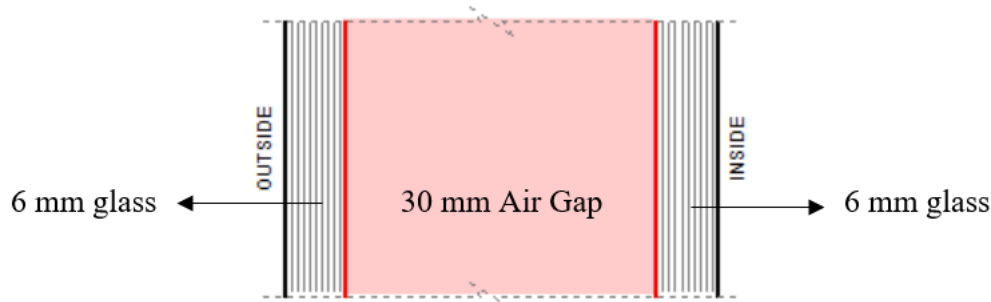
Figure 3.8 : Section of window and balcony door glasses.
