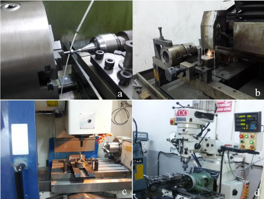
Figure 2.28: Manufacturing techniques which are used for production of transvaginal uterus amputation device. (a) Turning lathe, (b) Wire cut, (c) CNC, (d) Router.
