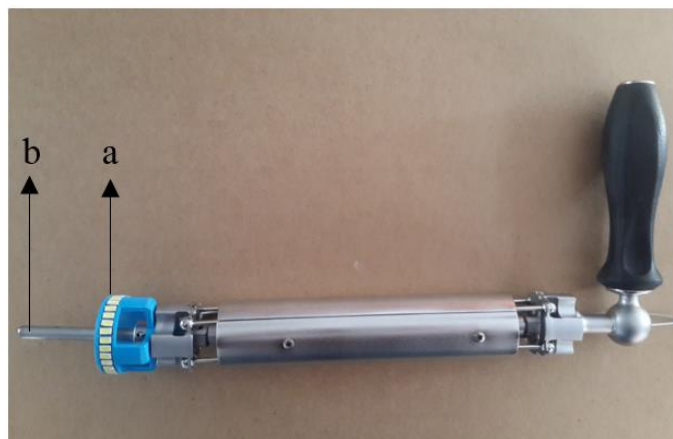
Figure 2.29: LED system implemented transvaginal uterus amputation device prototype made of stainless steel. (a) Cervical cap with LED illumination system, (b) Uterus tip.
