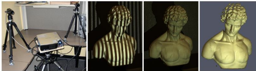
Figure 1.20: Structured light for 3D scanning. From left to right: a 3D scanner system with a pair of camera and a projector, two images of structured light on target object, 3D model of scanned object (Lanman D. and Taubin G. 2009).
