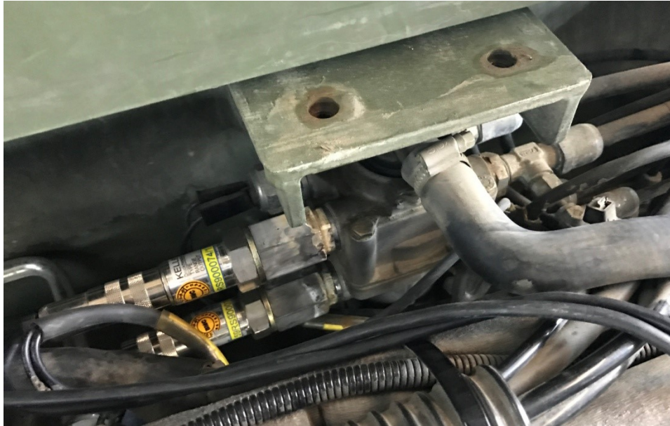
Figure 4.4 : Pressure sensors fitted on the foot brake valve.
