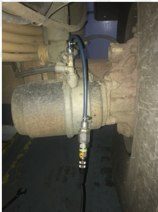
Figure 4.9 : Pressure sensor mounted on the rear axle left of prototype vehicle.
