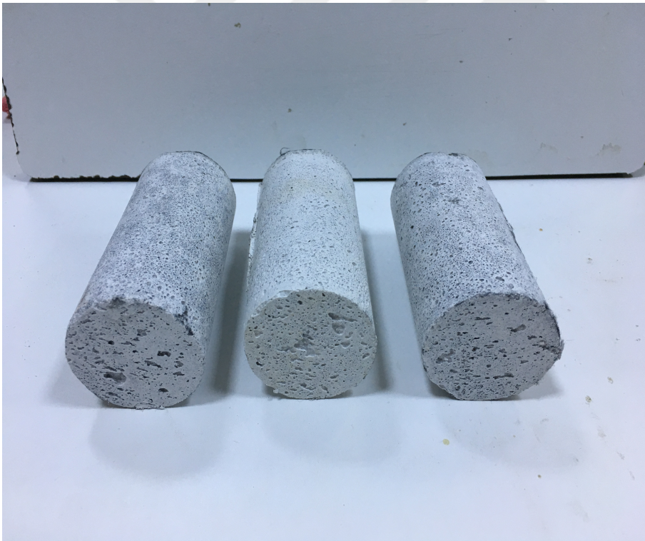
Figure 3.21 : Ø50x100 mm cylindrical samples for splitting tensile strength test.
