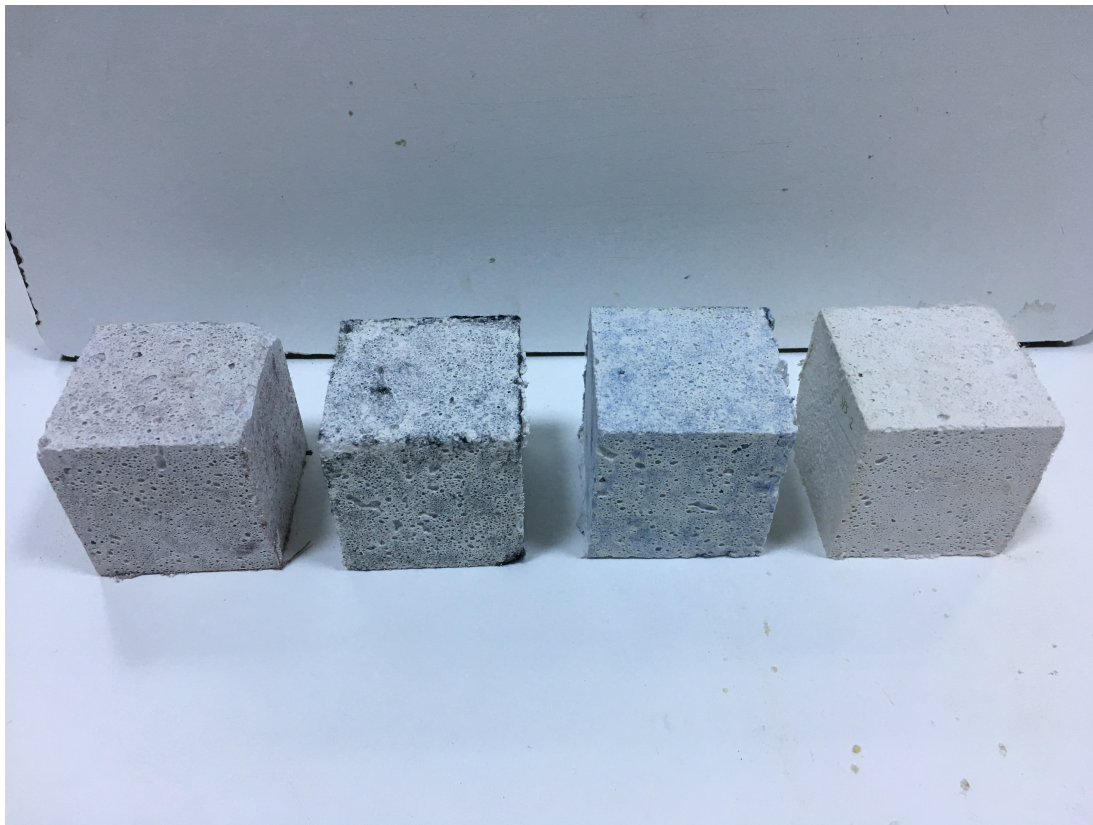
Figure 3.16 : 50x50x50 mm cubic samples for compressive strength test.
