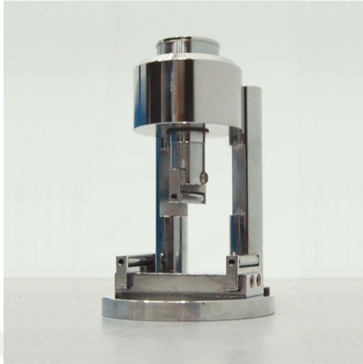
Figure 3.18 : Three point flexural testing apparatus (Url-7).
