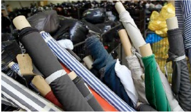
Figure 2.11 : End-of-roll textile waste is factory surplus textile waste leftover on the textile rolls from garment manufacturing (EcoChic, 2013).
