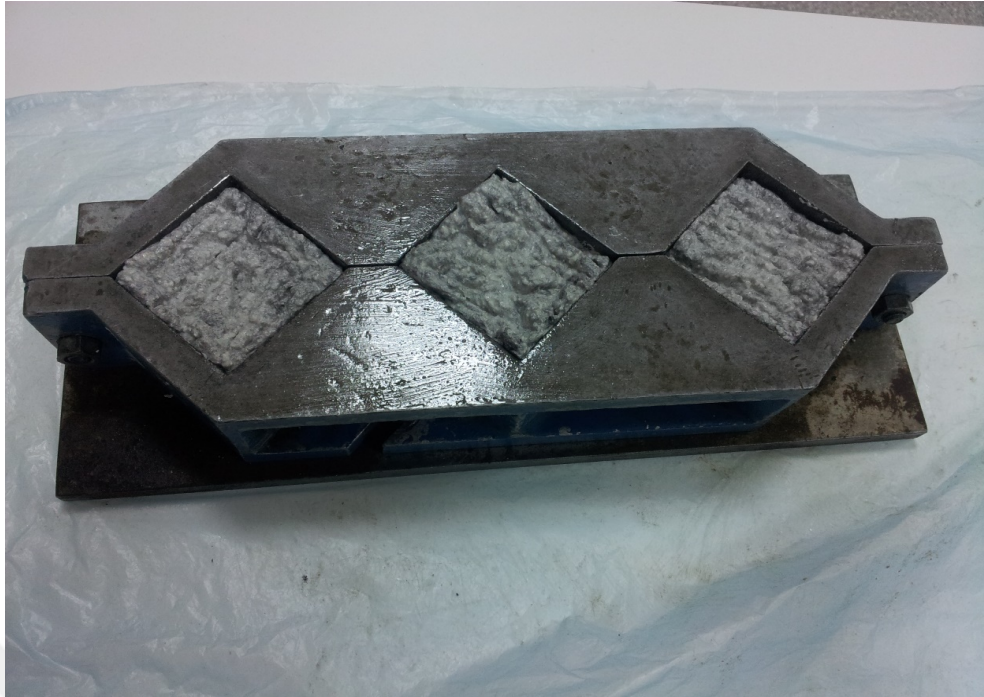
Figure 3.13 : Molding of the plastic mixture.
