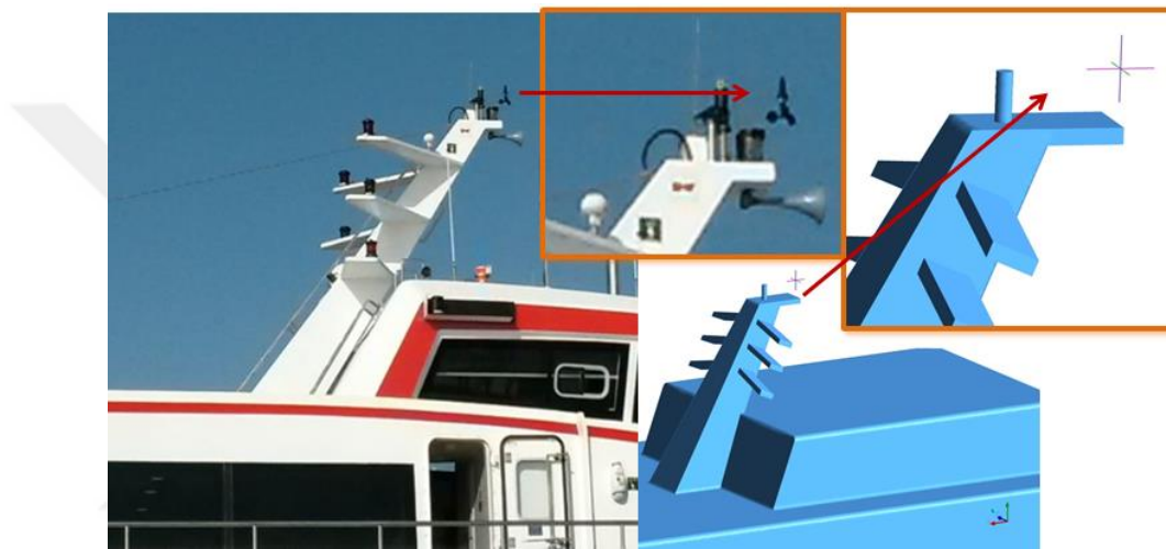
Figure 3.18 : Anemometer Sites and Details for the Real Catamaran Ship and The Model.
