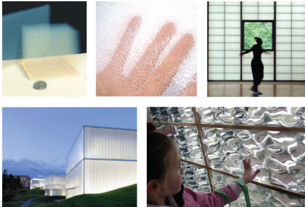
Figure 3.24 : Some examples of transparent insulation materials.
