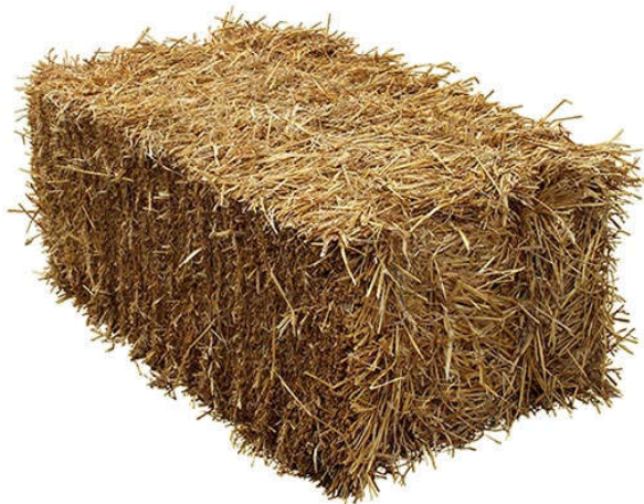
Figure 3.20 : Straw bale insulation pack for construction.
