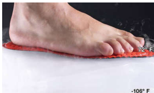
Figure 3.32 : An example of aerogel insulation dividing the cold from hot.
