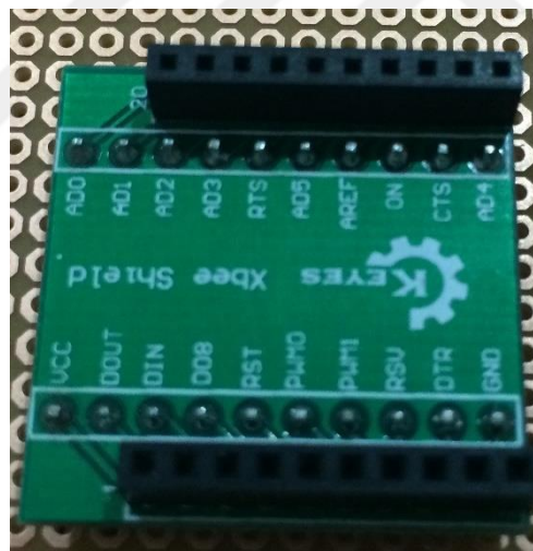
Figure 3.3 : XBee breakout board
