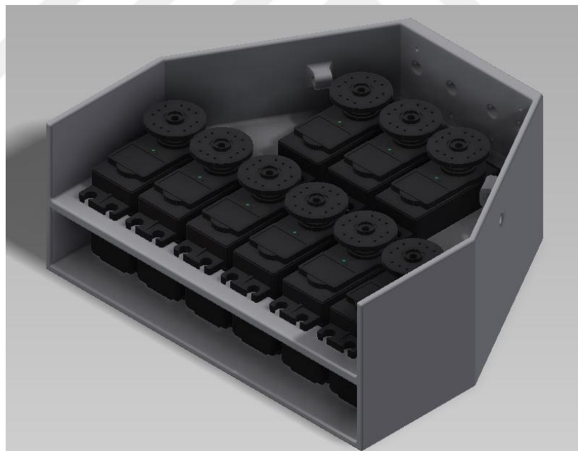
Figure 4.18 : Assembling of servo motors and wrist.
