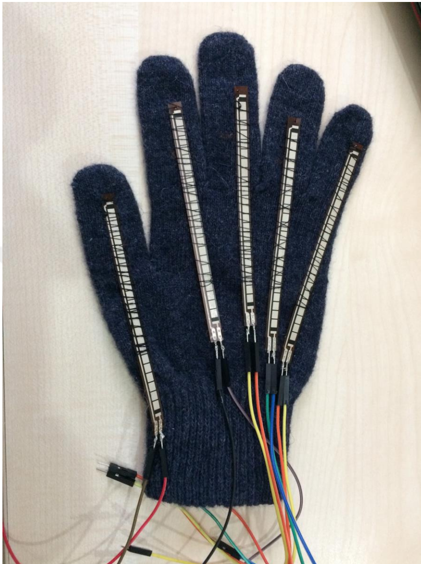
Figure 5.10 : Flexible sensors on gloves.
