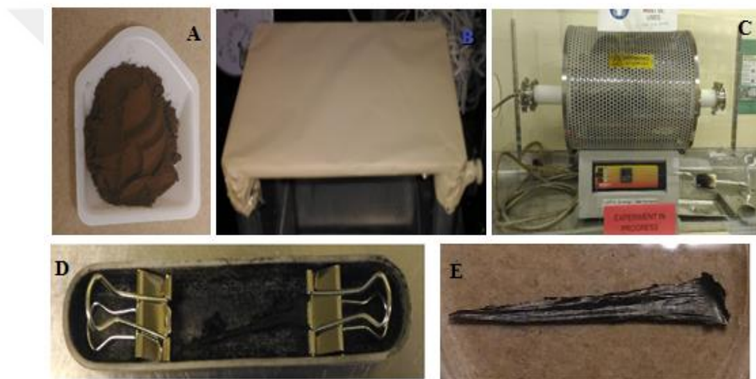
Figure 3.24: Sample preparation for thermal processing, (a) lignin powder, (b) electrospun PAN/Lignin nanofibers, (c) horizontal tube furnace (d) placement of carbon nanofibers in the ceramic boat after carbonization, (e) carbonized nanofibers.
