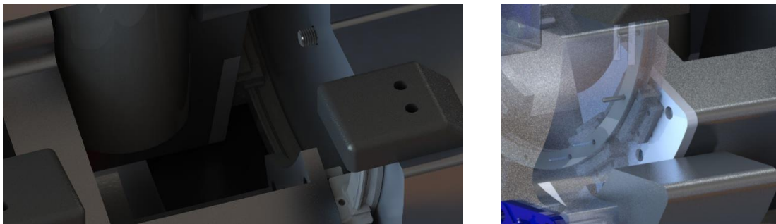
Figure 2.10: R-Guide rails connection with upper jaws a) Inside view b) Outside view behind the transparent base wall.
