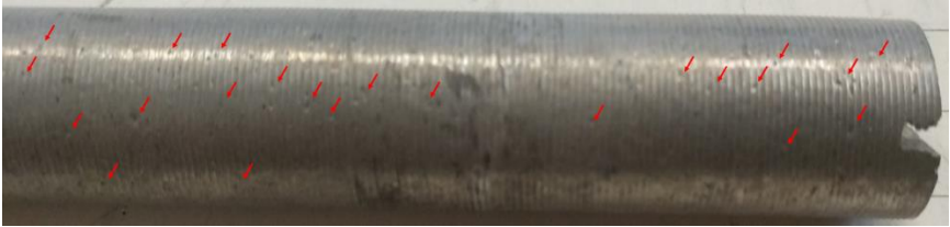
Figure 3.32 : The surface of a sample after HIP process.
