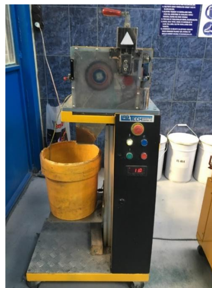
Figure 2.5: Product in spaghetti form Figure 2.6: Pellet machine
