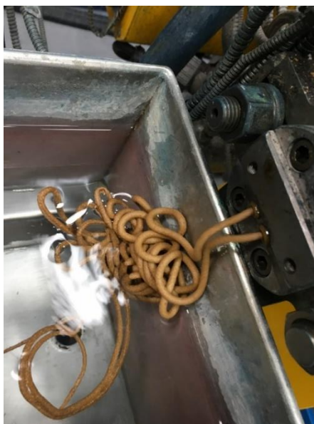
Figure 2.5: Product in spaghetti form Figure 2.6: Pellet machine
