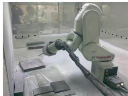
Figure 3.13 : Commercial LPCS equipment and automated spraying gun system [22].
