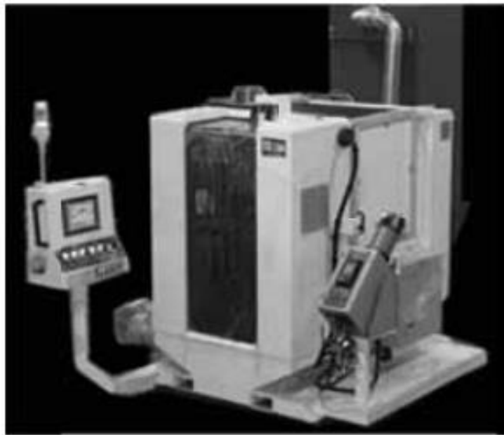
Figure 3.11 : Image of commercial stationary HPCS system [27].
