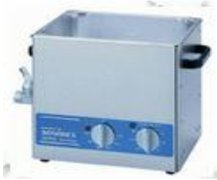
Şekil 5. 1: Ultrasonik banyo (Sonorex Ultrasonic Bath RK-100 H)
