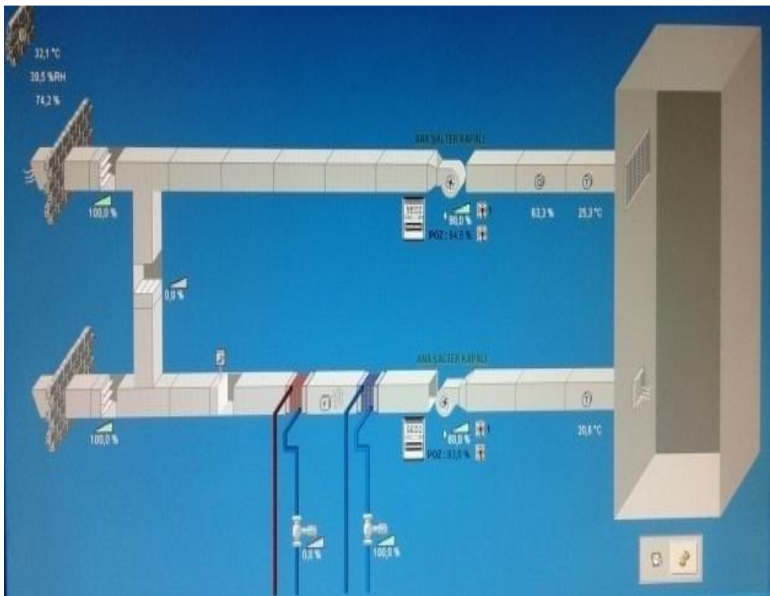
Figure 3.14: AHU 49 operating window without Solarwall system.
