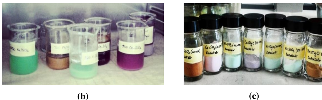
Figure 4-1 : (a) “Bandelin Sonoplus” sonicator (b) Catalysts during drying process. (c) Catalysts after grinding
