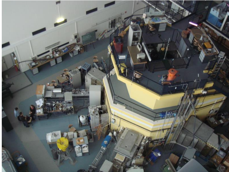
Figure 3.16 : TRIGA Mark II reactor of the Atominstitut [20].
