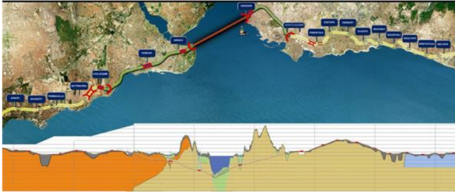
Figure 3.1 : Marmaray Project Plan and Profile [16].
