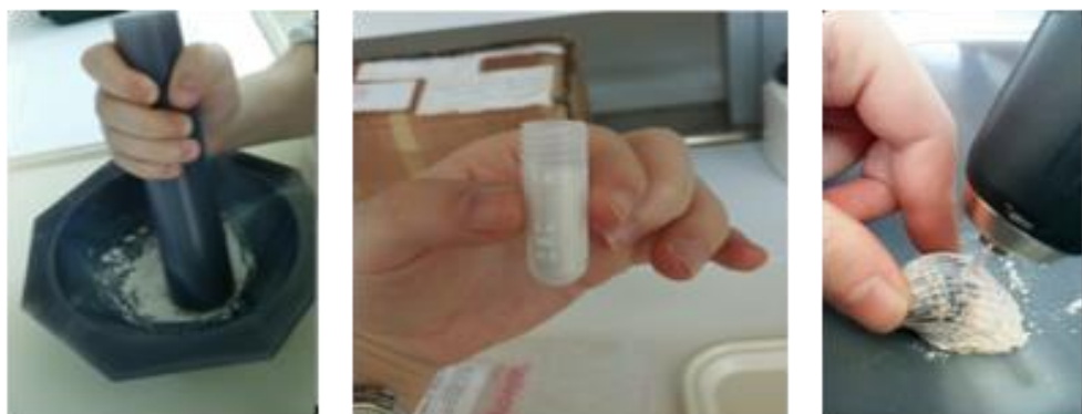
Figure 3.14 : Agate mortar. Plastic container and drilling
