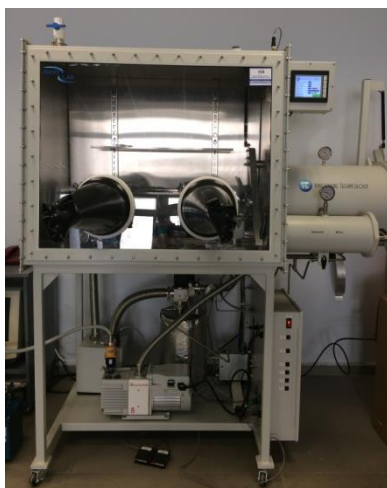
Figure 5.9 : Innovative technology IL-2 GB glove box.
