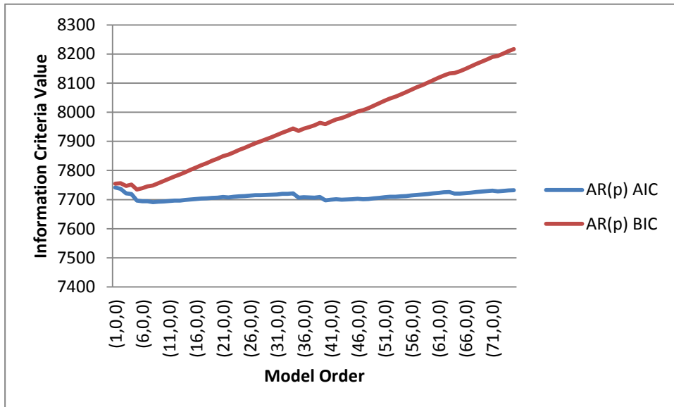
Figure 3.4: AIC and BIC results of AR models from AR(1) to AR(75).
