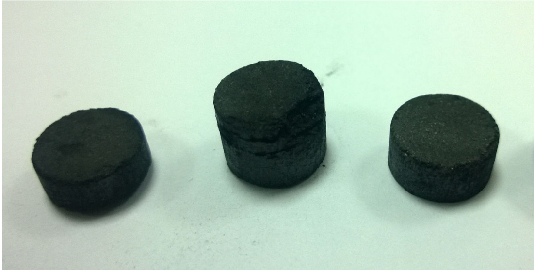
Figure 6.22 : 90% Coal slurry, 10% CPW briquettes.
