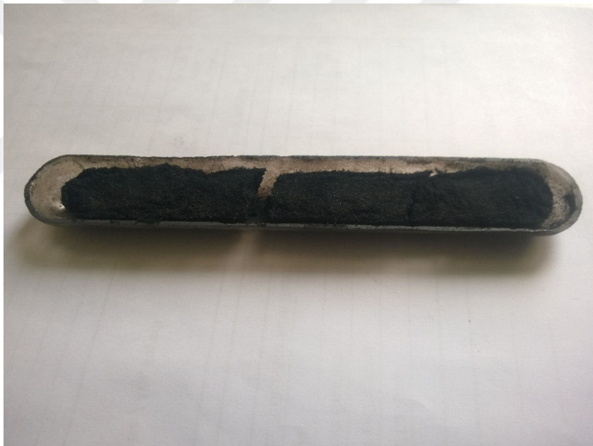
Figure 5.12: Carbonized MDF shavings.
