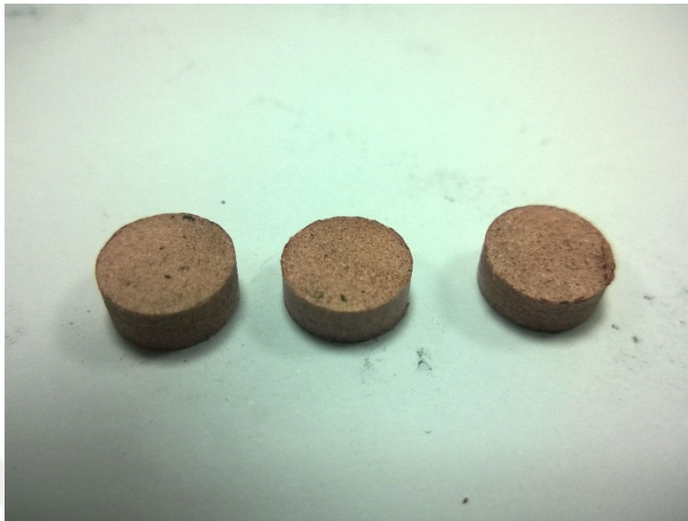
Figure 6.24 : 100% Pencil shavings briquettes.
