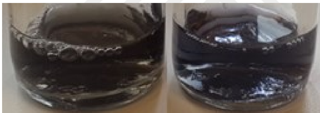
Figure 6.5 : Separated m- and s-SWCNT with Sephacryl gel (green-brown one is metallic and blue one is small semiconducting).
