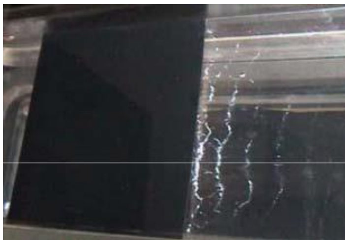
Figure 3.7 : Von Karman vortex cavitation, adapted from [81].
