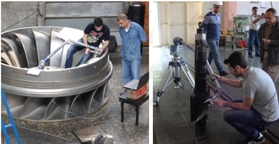
Figure 4.3 : Laser scanning studies in Kadincik I HPP.
