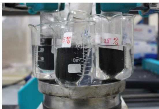
Figure 3.3 : The mixture is on the magnetic stirrer to complete the polymerization process fastly.
