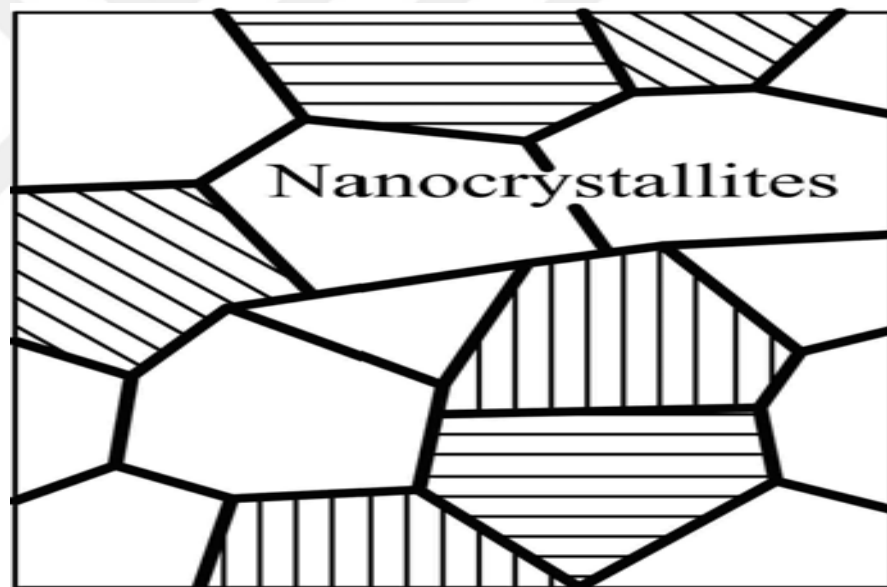
Figure 1.7 : The schematic structure of 3-D nanomaterials.
