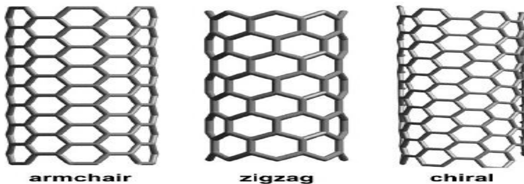
Figure 1.9 : Types of single-wall carbon nanotubes.
