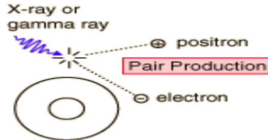
Figure 2.13 : The schematic view of pair production (Url-11).
