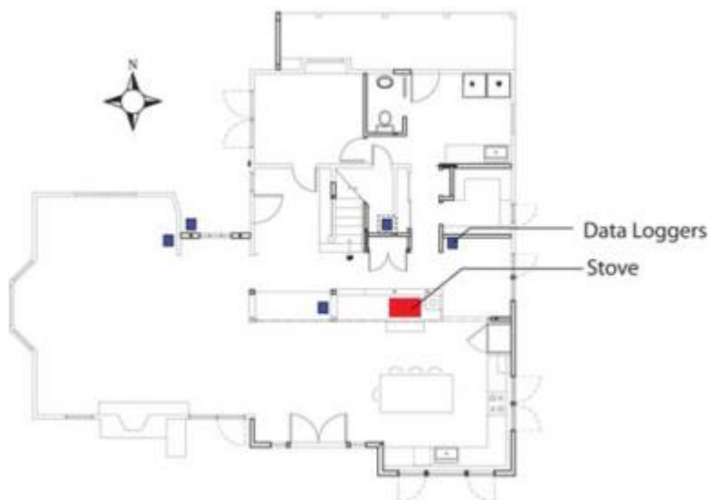
Figure 1.18 : First floor plan of the barkman residence showing the location of the contraflow masonry stove and data loggers (Hanley et al., 2005).
