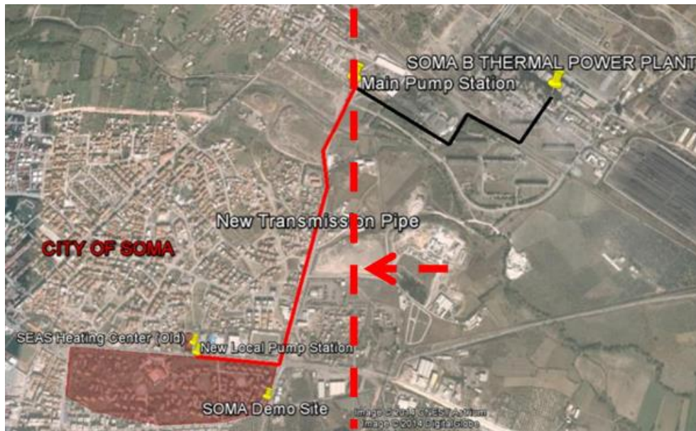
Figure 4.4 : New district heating system pipeline.
