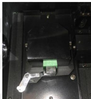
Figure 4.21: Placing the reflector in the device.
