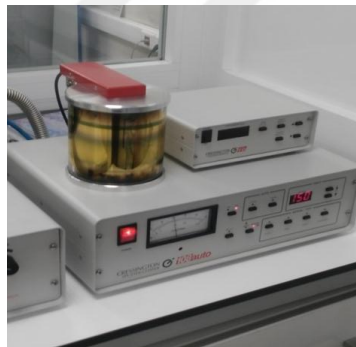
Figure 4.15: The process of coating the surfaces of samples with gold and then vacuuming of PMMA's.
