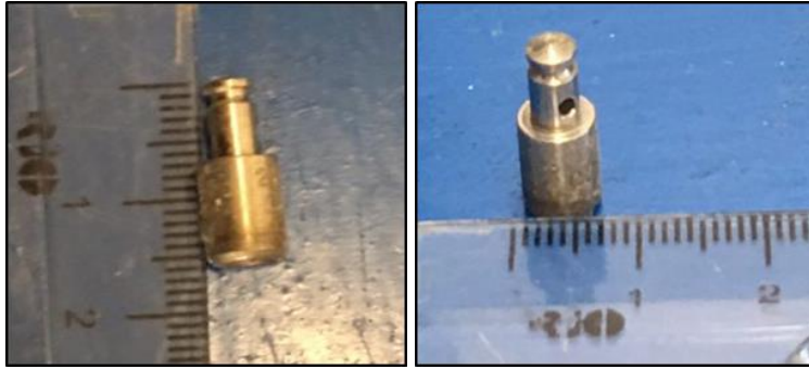
Figure 3.6 : Images of the Gamma source (Co-60 radioisotope).
