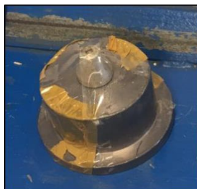
Figure 3.5 : The image of Gamma source (Cs-137 radioisotope).
