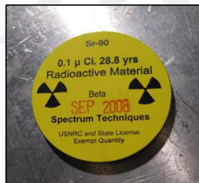
Figure 3.10 : The used beta source (Sr-90).
