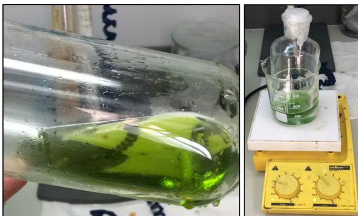
Figure 3.3 : The completion of polymerization process with magnetic stirrer.
