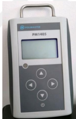
Figure 4.15 : PM 1405 Geiger- Muller detector as the measuring device.
