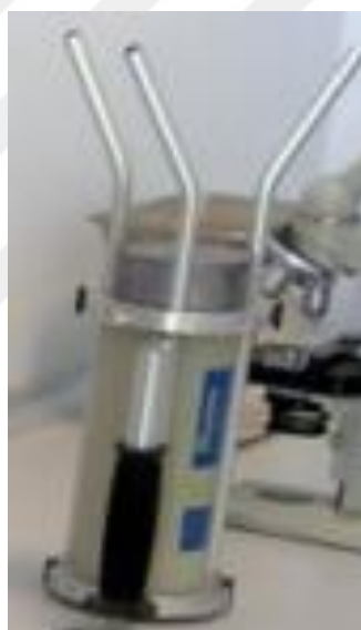
Figure 4.14 : The Sr-90 radioisotope source used in the beta counts was inserted inside the experimental setup.
