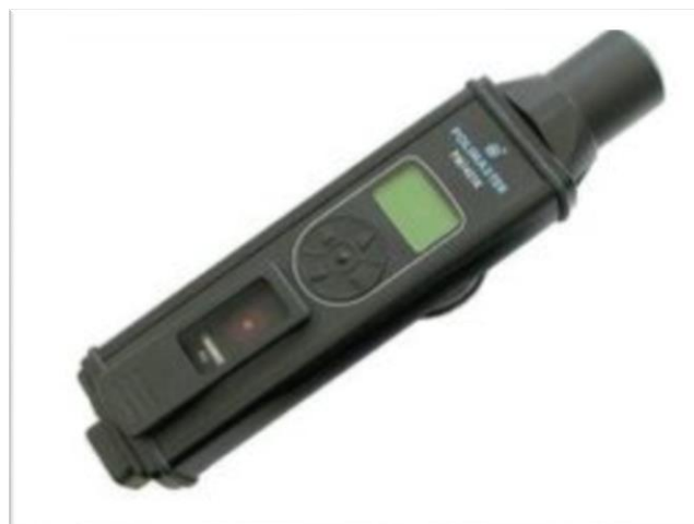
Figure 4.17 : PM1401K Model scintillation detector.
