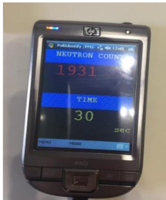
Figure 4.18 : Pocket PC that can work compatible with the scintillation detector.
