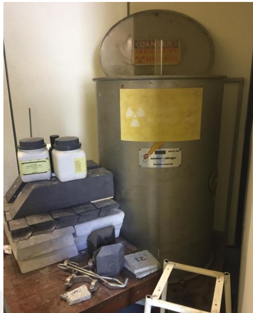
Figure 4.16 : Experimental setup of Pu-Be Neutron Howitzer for the for neutron transmission design.
