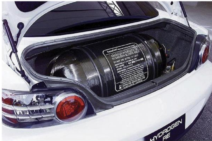
Figure 2.18 : Storage tank of a Mazda RX-8 Hydrogen car (Alaswad A, 2016).
