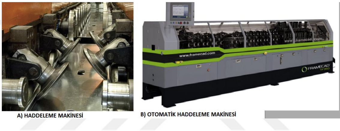
Şekil 2.3: A) Haddeme Makinesi (roll forming machine) B) Otomatik Haddeme Makinesi (Anonymous 2019a);(Anonymous 2019b).
