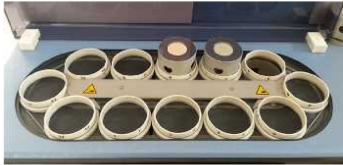
ekil 3.3.4 Thermo Scientific ARL 9900 WDXRF numune de i tiricisi
